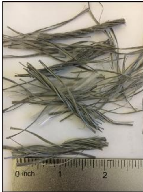
Figure 2: Photograph of the fiber used in MnROAD 2017 FRC research cells.
