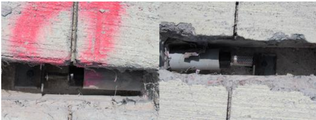
Figure 55. Sketch and photographs of joint opening sensors before installation of protective covering.
