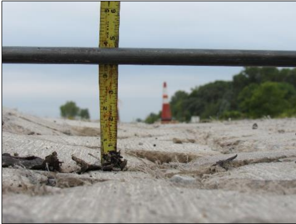
Figure 6. Depression along with the wheel path in Cell 139.
