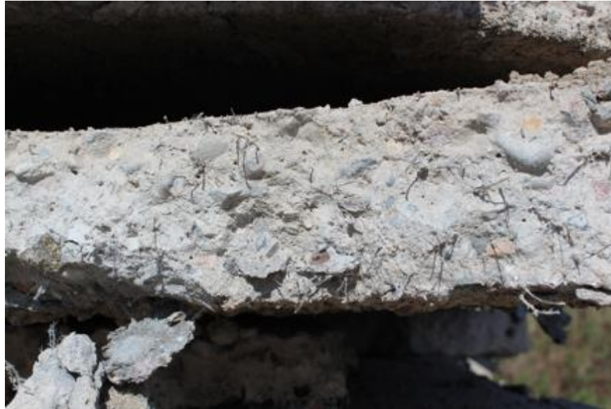
(7c) Fibers on the fractured face of a concrete piece.
